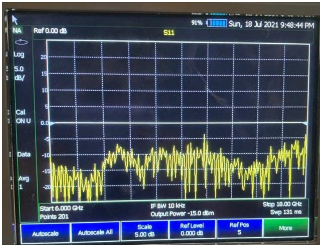
Return loss of 5 element linear array
