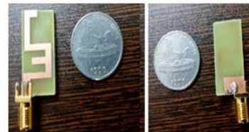
Fig 2: Fabricated Dual band antenna size comparison with a coin
