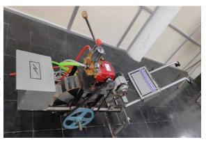
A small machine that can take up multiple tasks in farming is the idea for this project. The Multipurpose farming machine was designed and fabricated by the final year students of Mechanical Engineering Department with a support of Rs. 20,000 from the College. The machine can be used for tilling, ploughing, spraying pesticides and fertilizers, pumping water to the farm seamlessly. The machine uses rechargable battery as a power source and works for an hour per every hour of charging
