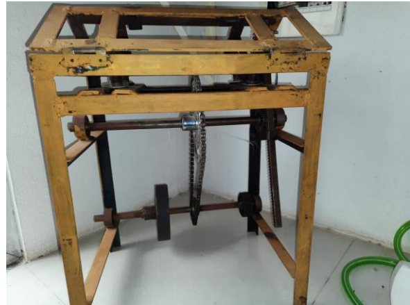
Fig. 2. Power generation through shock absorbing mechanism.
