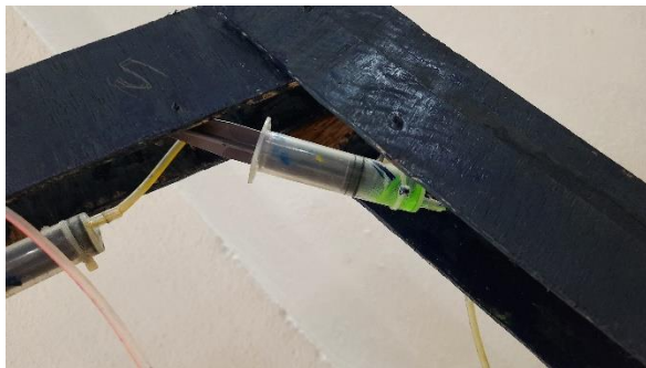
Fig. 2. Joint powered by hydraulic pressure from syringes.
