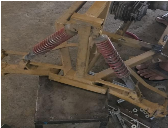
Fig. 2. Double wishbone suspension system The braking system is composed of both internal expanding drum brakes and disc brakes. The drum brakes are installed at the two front wheels and a single rotor is mounted on the rear axle to satisfy the braking requirements of our quad bike such as terrain of the track, speed limits, driver ergonomics and other rulebook constraints. The front drum brakes are mounted on each wheel of internal radius 2.5 inches having a brake lining width of 3 mm. The distance between the pivot point of both the brake shoes and the cam is 3.93 inches.
