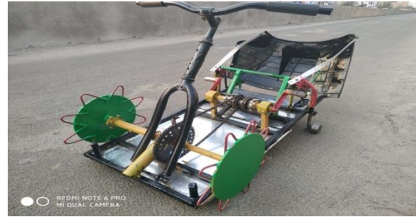
Fig. 3. Working Model of the Rice Transplanting Machine
