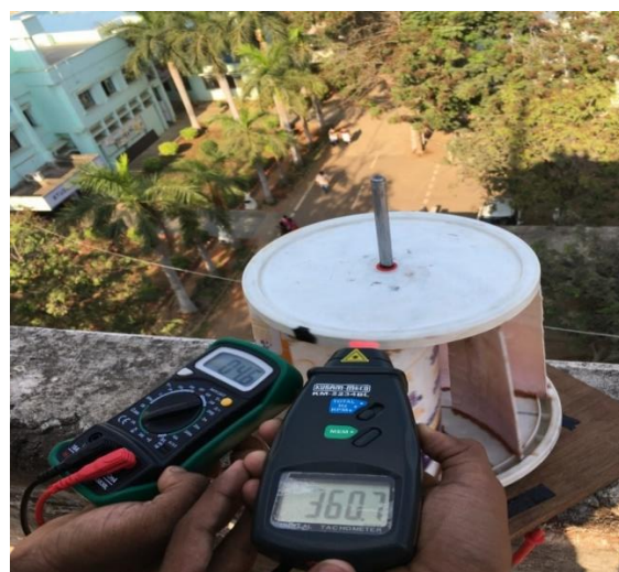
Fig. 2. Working of Maglev vertical axis wind turbine
