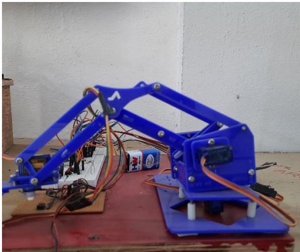
Fig. 3. The Robotic arm with controller circuit.
