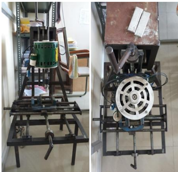
Fig. 2. Assembled view of Friction Stir Welding Machine.
