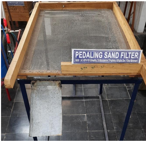
Fig. 1. Filter used for filtering the sand.
