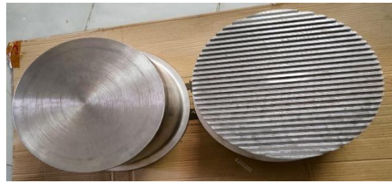
Fig. 4 Cooking pot with and without fins
